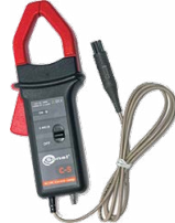
C-5A clamp ( \Phi 39 mm) 1000 A AC/DC
